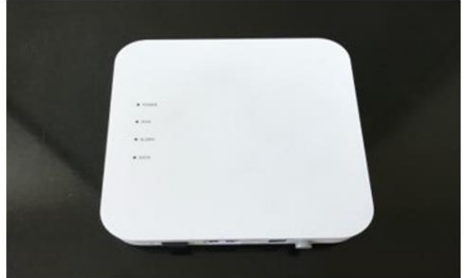
Figure_23: NBI Optical Network Terminal (Nokia xsXS-040x010X-AQ )
