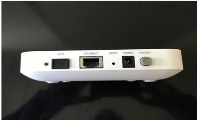
Figure_23: NBI Optical Network Terminal (Nokia xsXS-040x010X-AQ )
